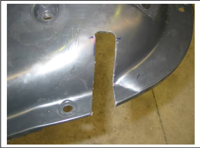
Figure 3: Trimmed under body guard, removed from vehicle for photo.
